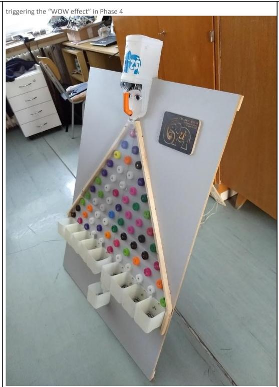
It is also advisable to cover a large area (especially in the upper part) with plexiglass or something similar - to prevent the marbles from popping when dropped at high tilt. With a small tilt, this is not necessary - it is necessary to keep this in mind when catching the marbles - when the marble may not have enough energy to "skip" the rim of the cup. Anyway, it is up to the teacher / students to think about it in Phase 2.
